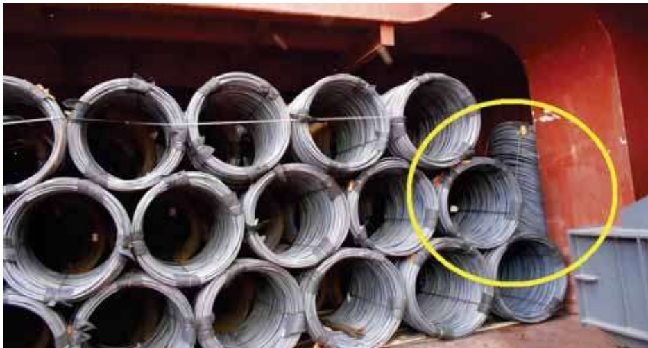
✘ One coil has fallen off the stow and is sitting vertically, and unsecured
