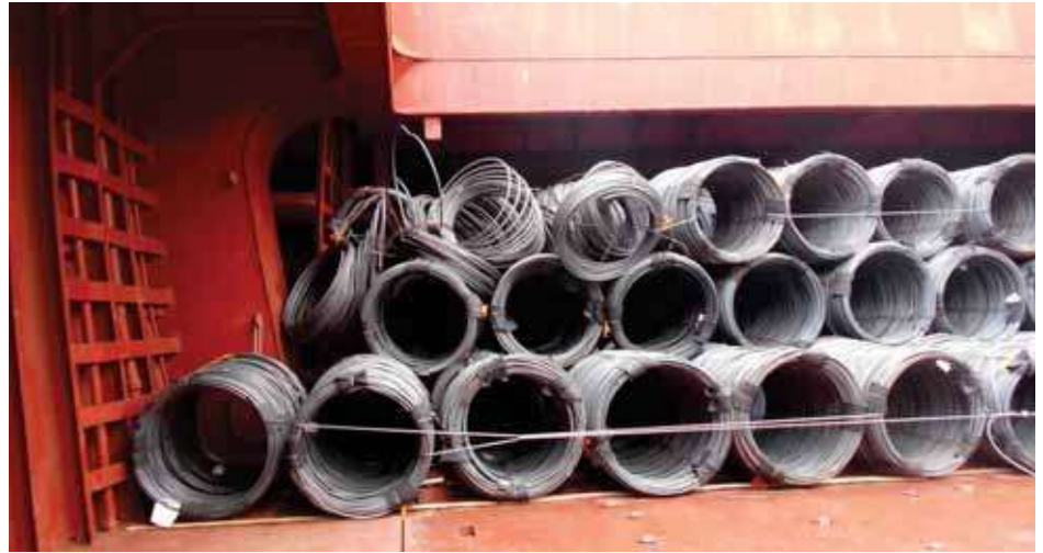
✘ The stow of coils is not tight across the hold due to the unwound coils
