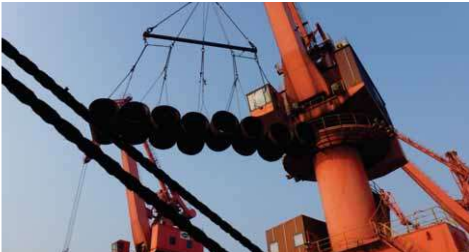
✘ In this set-up, 8 coils are loaded. However, the slings are made of wire. This is not recommended as it may damage the coils or their securing straps/wires
