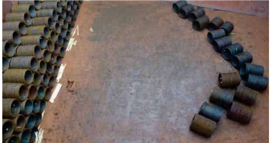
✘ Poor loading practice. Coils landed directly onto a tank-top covered with previous cargo residues. The cargo residues may react with the steel
