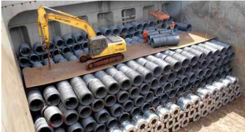
✔ Completing a stow in the aft part of the cargo hold. The forward-facing vertical wall will need to be lashed
