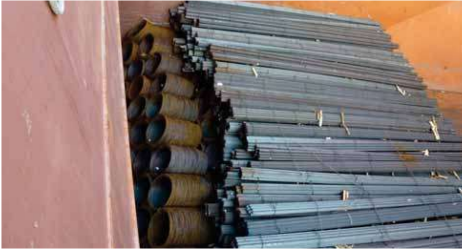
✘ Lengths of structural steel stowed on top of coils. The WRIC stow collapsed and had to be offloaded. Many of the coils were damaged
