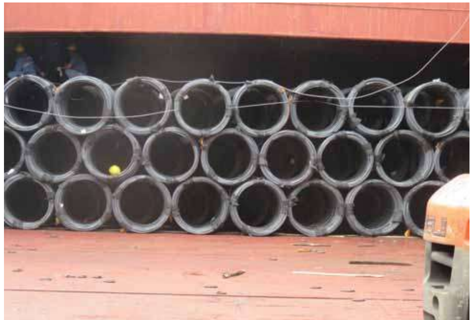
WRIC loaded in the 'tween deck space. The lashing gang are securing the top tier of the face of the stow
