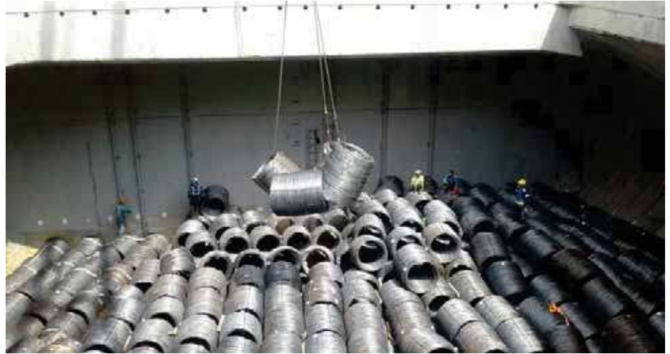
✓ The coils will be offloaded by a single leg basket through the WRIC. 4 WRIC handled with 2 wire slings
