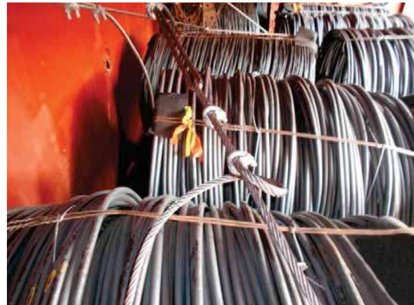
✘ Incorrect use of bulldog grips with grips on the live wire. Insufficient number of grips used
