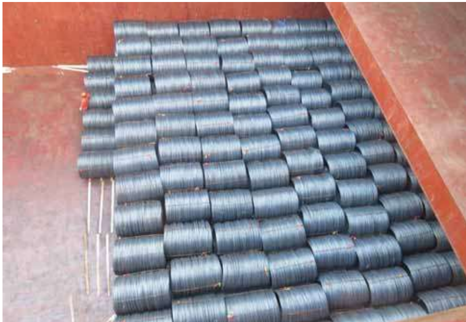
WRIC being stowed across the full width of a box-shaped cargo hold
