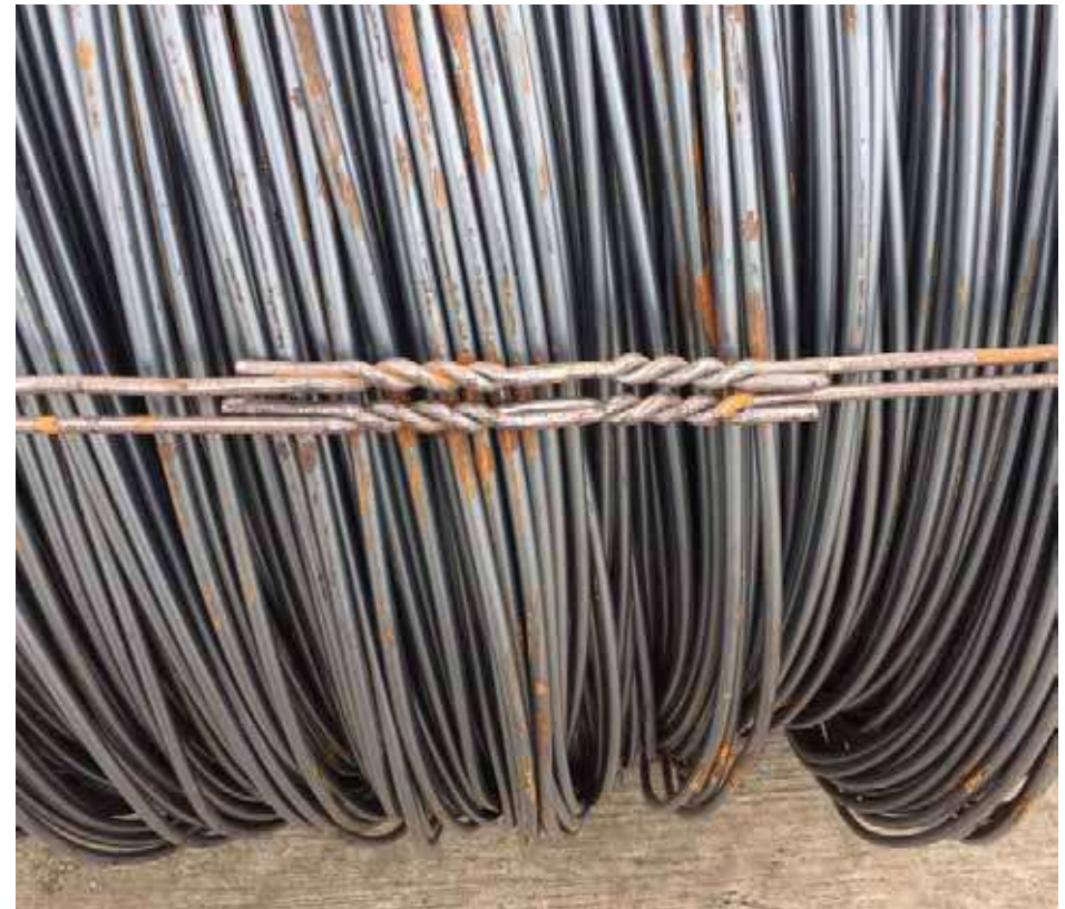
Bundling of WRIC with the use of double bundling wire rods and four twists
