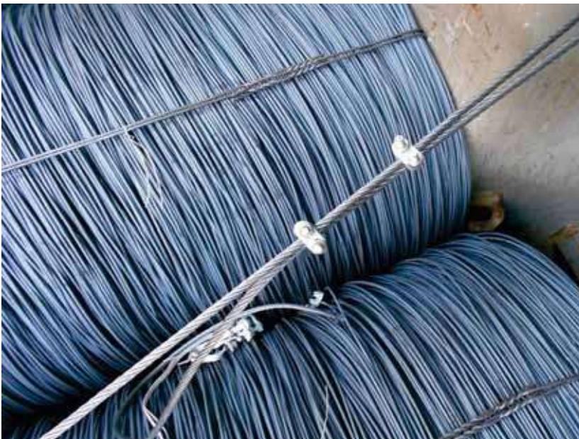
✘ Incorrect use of bulldog grips
