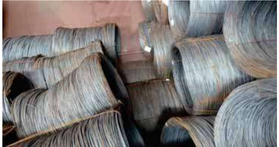
✘ Poorly stowed outer coils in a bulk carrier. Although the tiers are lashed, the outboard coils are leaning forward and will likely collapse on the voyage
