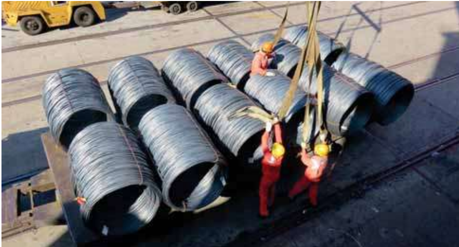
✔ Slinging the coils for loading. One nylon belt per coil is used to avoid damage to the cargo
